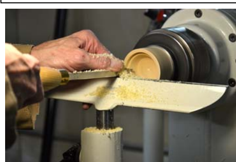
9. Cutting the recess for the box bottom. He's using the Bedan tool to make a square shoulder.
