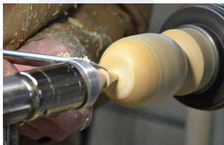
12. The top is nearly shaped, leaving a cone to be carved into a stem.
