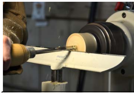
5. The lid is re-chucked & hollowing starts.
