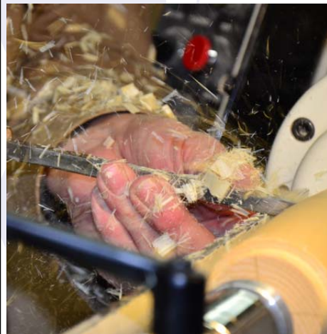
1. Using a Bedan tool to make a tenon on each end of the piece.
