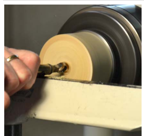
7. The proper angle for using the ring tool.
