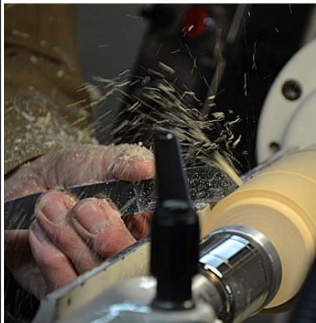
4. Parting off the first piece with a very narrow tool, which helps keep grain matching.
