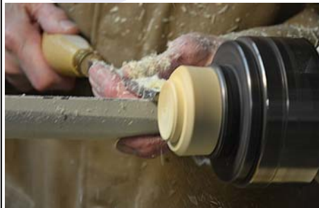
14. Forming the waste into a jam chuck.
