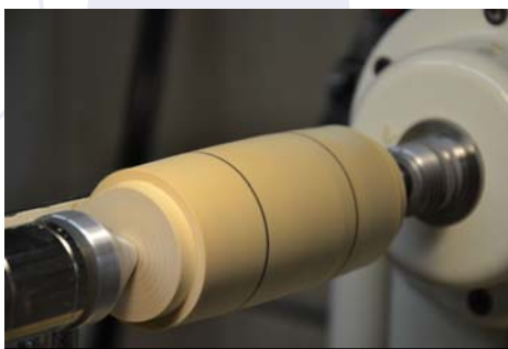
2. Marking off 3 sections of the project. Left, the box top. Middle, the bottom. Right, waste piece to be used as a jam chuck.
