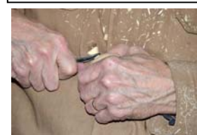
13. Shaping the bottom & parting off the waste.
