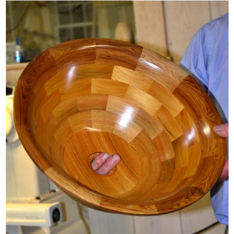
Russ's hand sink bowl. It's made from cedar wood out of a brewery. It fits under a standard-size sink top cutout.
