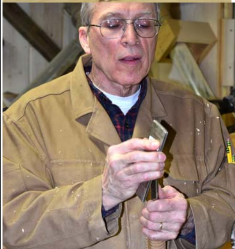
(Left) Ted hones his skew chisel, which he finds the fastest way to rough out a project with grain aligned with the lathe.
