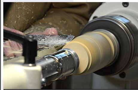
11. The top is jammed onto the bottom, and shaping starts with the skew.
