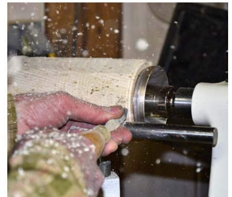
Step 8. Defining the lip, using a large cone tailstock.
