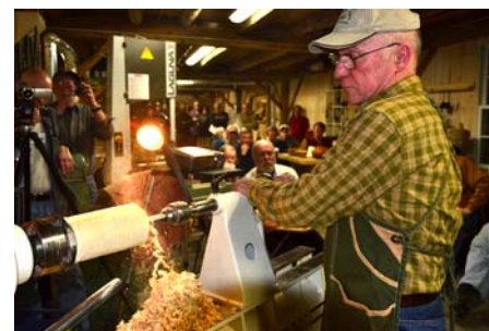
Using a story stick to measure length of cup.
