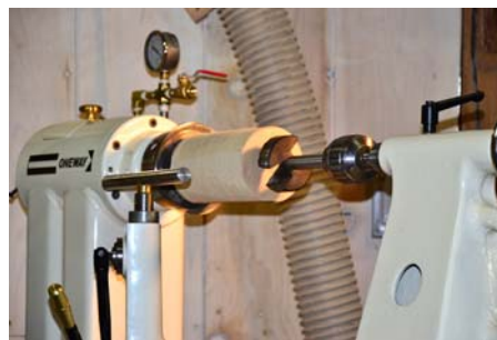
Step 5. Drill hole with Forstner bit.
