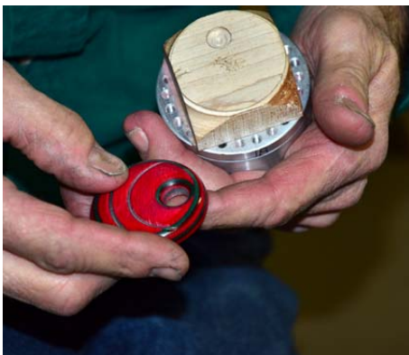
Mike Perron shows small chucks to hold small works.
