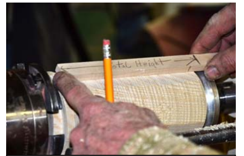
Using a story stick to measure length of cup.
