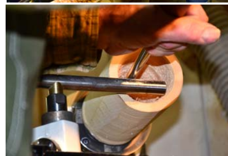
Steps 5 & 6. Drilling, then hollowing.
