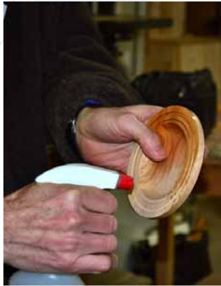
Prepping the surface with shellac.
