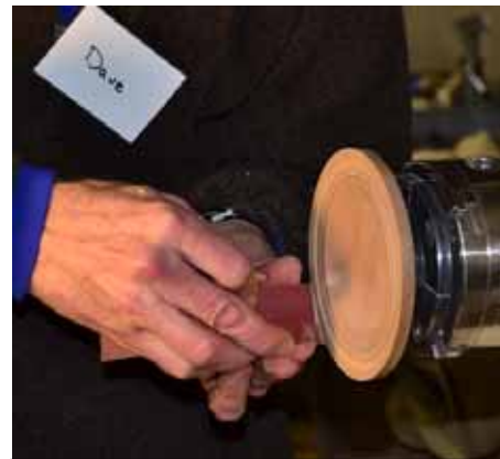
Cutting & sanding the grooves.
