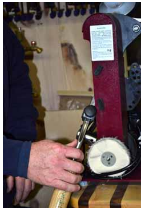
This is Bill Walsh's Sorby belt sharpener, modified to do a side grind.
