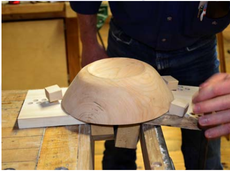
Greg Drew demonstrates his invention of a vice to hold bowls for sanding once off the lathe.
