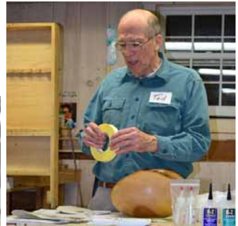
Ted had a problem when the bark separated after drying. The bowl contracted differentially along its axes. This stretchy, sticky tape allowed re-attaching the bark.
