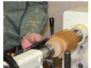
Ted demonstrates the rounding cut, which is faster & smoother than using a roughing gouge.
