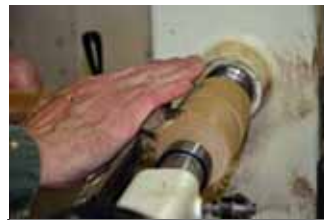
Finishing cut—fine hairs coming off the skew.
