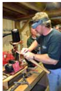
Putting on a fine edge with the Sorby Pro-Edge .
