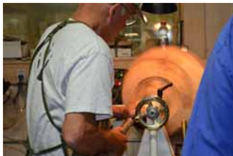
Russ chooses a center point by fastening a false bottom to the piece with hot glue and to the faceplate with strong screws. Don't use wallboard screws as they are brittle.
