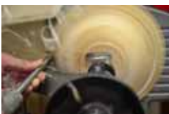
Drill a 3/8" hole in the center of the bowl top. Mount to a screw center & shape the outside, forming a spigot for reverse mounting.
