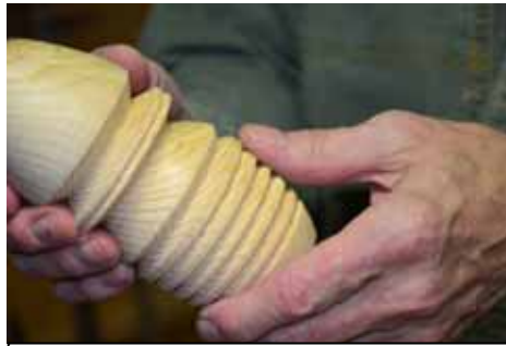
All these cuts are possible with a sharp skew. They can be smooth enough to avoid sanding.
