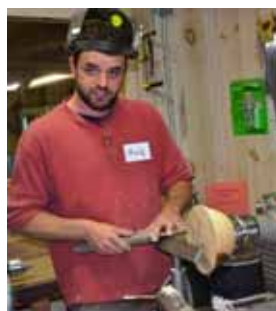
Mounting the bowl bottom to a scroll chuck, start shaping the center, using the tool so the edge, not the tip, cuts.
