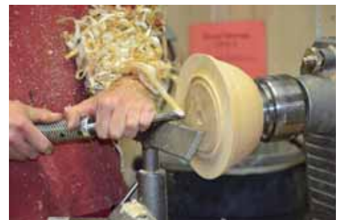
Nick is cutting from near the center outward with this cut. He will deepen the cut and get closer to the center as the bowl gets deeper.
