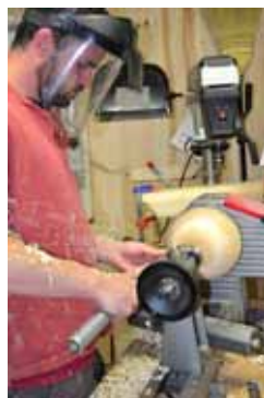
Nick shows the proper position & tool angle for a smooth exterior.
