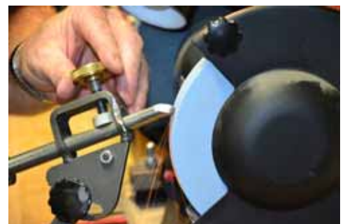
Putting an edge on a bowl gouge. This profile is similar to the Ellsworth grind.
