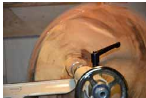
Russ has shifted the false bottom on the faceplate and is making a second cut. For safety, lathe speed should be slow enough so vibration is minimal. Always use the tailstock as long as possible,
