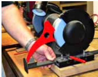
Setting the Oneway jig using a Raptor angle guide.
