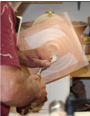
10. The piece has been reversed onto a vacuum chuck. The tape is to seal pores for a better grip. Al is finishing the foot and giving the outside of the bowl some interesting cove cuts.
