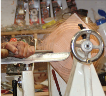
4. Rough shaping the bowl bottom. Al is using the ear of a bowl gouge.
