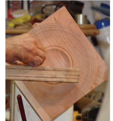
9. Al pencil scribes concentric circles and radial lines with random spacing.
