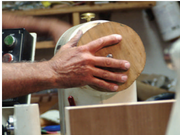
1. Mounting a spacer to a screw chuck. A matching hole (3/8") is drilled centered on the face of the blank.
