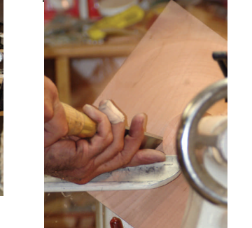
5. & 6. Al uses a flat-ended scraper ground to a sharp edge and used as a shear scraper to finish the bowl side. Note how the tool is held. A rounded corner is on the tool rest in a strong grip.
