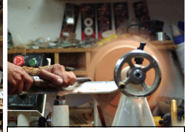
7. The piece is now held by its foot in a scroll chuck and the face is being refined. The bowl will have a shallow broad rim.
