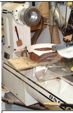
11. Resting on the bed is Al's large vacuum chuck. It can be mounted on a carving vise or to a wall to hold work at a comfortable angle.
