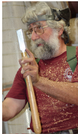
4. Rough shaping the bowl bottom. Al is using the ear of a bowl gouge.
