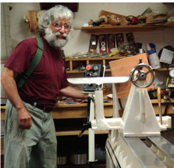
2. The blank is mounted and the tailstock brought up for safety.
