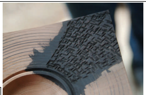
14. After drying, Al uses a scrubby to burnish the paint which reveals some of the wood.
