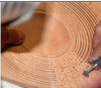
12. Making random-looking cuts with a high-speed tool.
