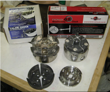
Top: Talon with #2 jaws. Nova G3 with Talon #1 jaws Bottom: Talon #3 jaws Nova #2 jaws
