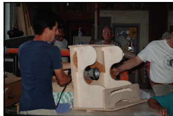
Here's Ralph inserting the router into the jig designed with SketchUp
