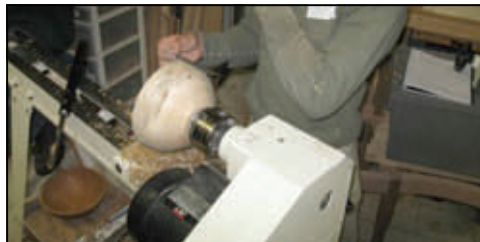
Reverse the bowl, tightening the scroll chuck properly. Be prepared to re-tighten.
