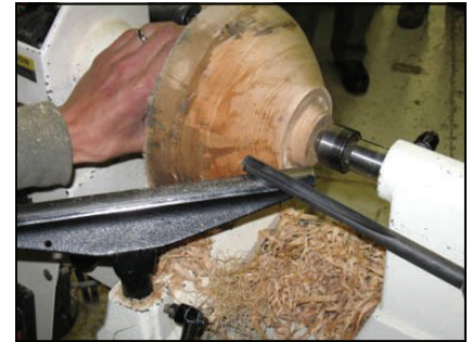
Form a tenon on the bowl base to fit your scroll chuck.
