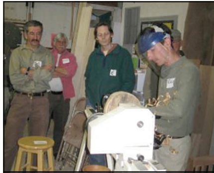
Bring up the tail stock for safety. Start shaping the outside of the bowl.
