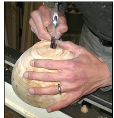
Use a very sharp chisel or carving gouge to remove the last of the tenon.
