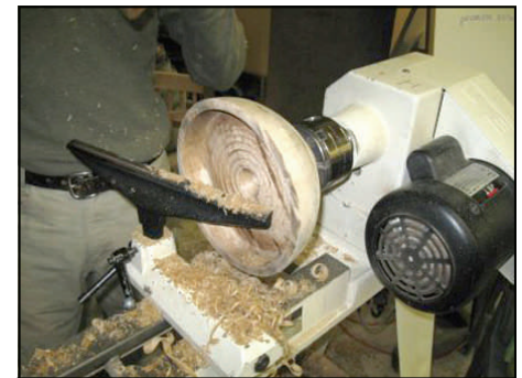
Hollow out the inside. Leave thickness about 10% of diameter.
