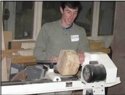
Bore a hole, usually 3/8" in the face side to accept a screw chuck..
