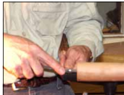
Continue cutting and allowing the tool to run into the work piece until threads look deep enough. Wax can be used to
