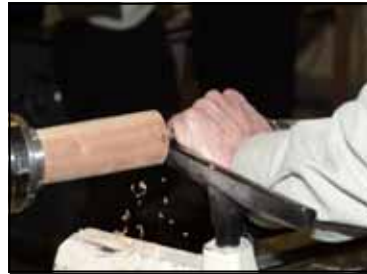
2. Set the lathe to its lowest speed. Begin at the outer edge with the tool tilted horizontally.
