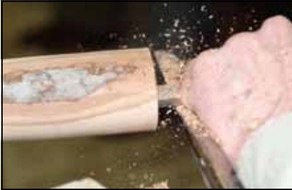
1. Cut a recess in the body of the box. Sides should be parallel. Leave enough wall thickness.
