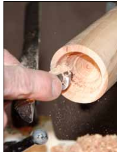
Looking at the cutting action from the back side of the lathe. Notice that the arm rest is pulling the tool into the cut.
