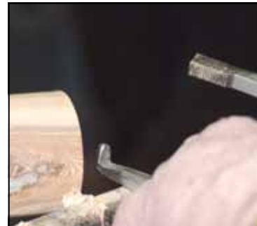
3. The arm rest is used with the thread chaser to bring sideways pressure on the tool. Pull toward you and let the tool travel into the work.
