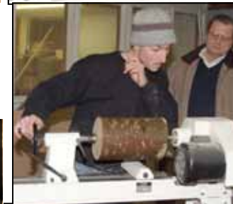
Typically, an end grain turning starts with a limb or segment in which the grain direction is between the headstock & tailstock.
