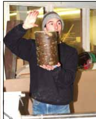
The length of the stock is reduced to pleasing proportions and the tenon is sized for the chuck.
