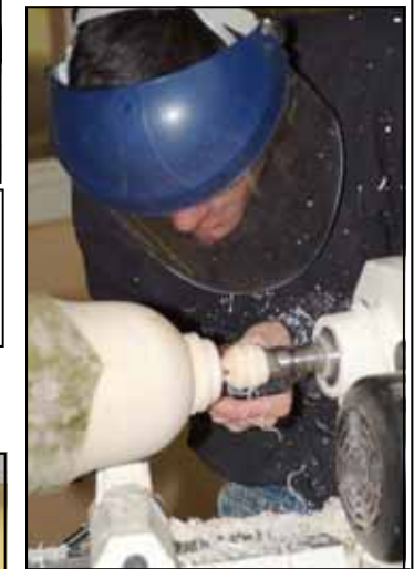
The length of the stock is reduced to pleasing proportions and the tenon is sized for the chuck.
