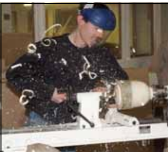
The hollowing process is started. Until the inside edge of the object is defined, the tailstock is used as a safety measure.
