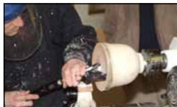
The tailstock is pulled back and the inside form is worked on with a hook tool or ring tool.
