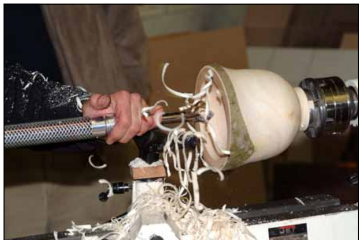
Continue hollowing with the hook tool. On a green piece, leave about 1" thickness & put aside to slowly dry. Re-turn to final shape/thickness.
