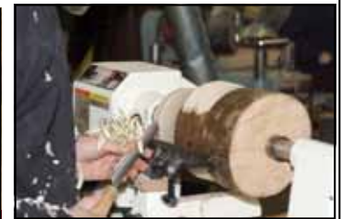
An early step is to form a tenon which can be gripped by a sturdy scroll chuck.
