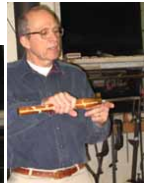
Ted—Heavy scraper with long handle; Roughened tool handles – not smooth; aids with grip / less fatigue when used for long periods of time and Jig to cut block from bottom of bowl
