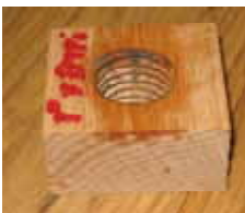
Bob Bouvier Piece of Oak tapped to thread on to lathe spindle – 1" x 8 TPI
