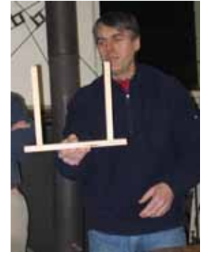
Craig Hall—Simple jig to hold spindle pattern
