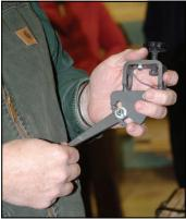
4. The Vari-Grind jig (Craft Supplies #130-4150, 48.99), is a versatile tool for a variety of grinds on bowl & spindle gouges.
