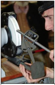
Ralph starts setting the gouge & jig up to copy an existing setup. With the jig angle at a guessed position, he moves the base arm until the side angle of the gouge rests fully on the stone. He then sets the angle of the jig arm so that the stone and nose angle match. Repeat as necessary so both the arm length and jig angle duplicate the desired grind.
