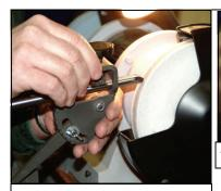
5. The Vari-Grind, together with the Wolverine Sharpening system, (Craft Supplies # 130-4100, \$85.99) produces excellent stability and a repeatable profile.
