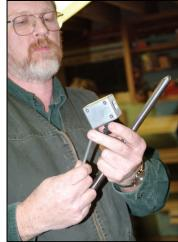
3. The Ellsworth grinding jig.(Craft Supplies # 066-0160,\$44.99) sets up for a good side grind on a bowl gouge.
