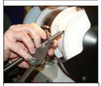
6. Rocking the gouge over to the left side, maintaining control to get a smooth curve from end to end of the cutting edge.
