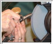
Now shape the gouge and put the proper edge back on it.
