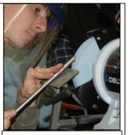
"Truing" the arc of the cutting edge. Lay the gouge flute side down on the flat guide. Bring the nose of the gouge in contact with the rotating stone. GENTLY, pull the tool toward yourself, allowing the stone to grind down the uneven curve, a little at a time.
