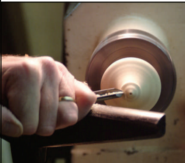
16. Finish the top & drill a small hole for the hanger.
