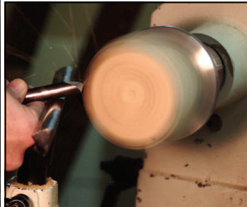
10. Starting to work on the top of the birdhouse. A block is attached using a modified screw chuck.
