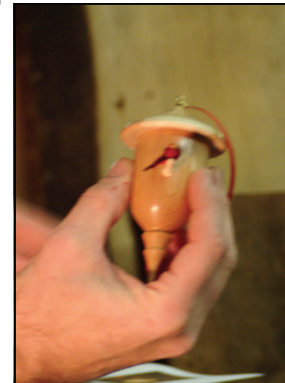
18. Finishing steps: Drill a nest hole & perch hole. Either turn a perch or use small dowelling. Sand parts separately, then Superglue together. Tie a ribbon onto the hanger, mount a teeny bird, and you are done.
