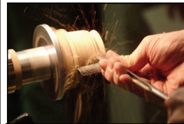
13. The top is reversed onto a pin chuck and its outside brought to shape.
