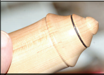
8. The tip is shaped. Here's a little optional wire-burned decoration.
