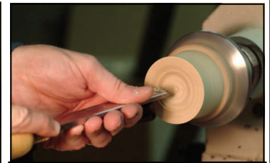
11. Working on the inside of the top. A recess is cut to the size of the body for a snug fit.
