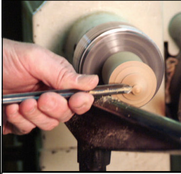
9. The piece is reversed onto the pin chuck and final detail work & sanding done on the body.
