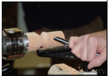
5. Putting detail on the outside before hollowing.
