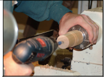
4. Drilling a hole to depth to begin hollowing out. This can be done using a chuck-held bit with lathe turned on. The tail stock is off for better access while hollowing.
