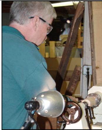
1. Turning a cylinder for the body. Cherry works well.
