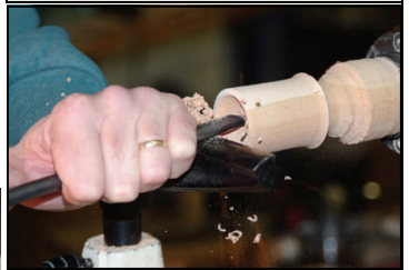
6. Traditional hollowing technique.
