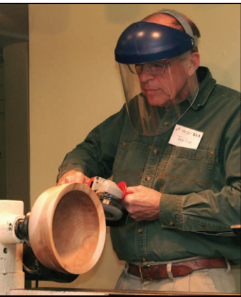
2. He's on the "wrong" side of the lathe. The work has to rotate away from the turner & this lathe doesn't reverse.
