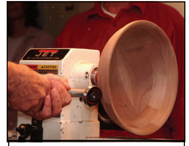
3. Russ using the Kutzall tool. This tool is loud, powerful, and requires a very low lathe speed for best texture.
