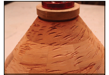
4. The results on a lathe turning at 500 RPM. A much slower speed would have produced closer marks.
