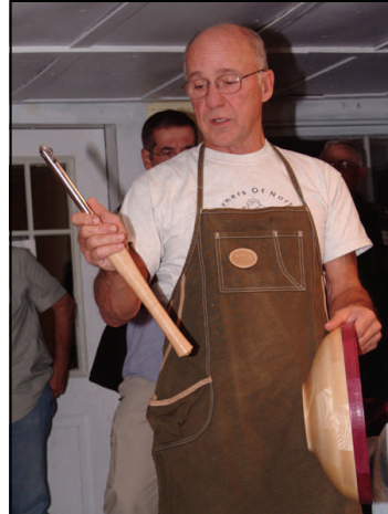
1. Russ generally uses the Sorby texturing system especially on his basket series of bowls.
