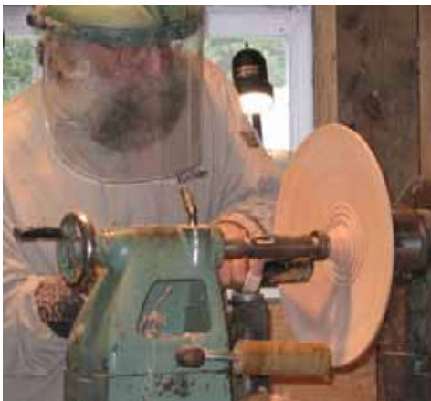
Taking down the rim to thickness. Get the rim thin before moving inwards to keep as much stiffness as possible under the gouge.
