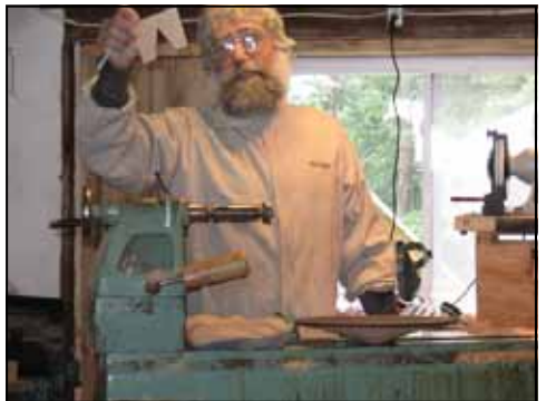
A very simple template is used to put a design on the surface. Al uses a watercolor pencil to put the design on the gesso. It is easier to erase its marks if you miss with the gouge.
