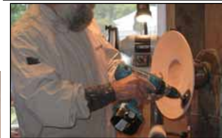
Final sanding of rim before applying surface coat.
