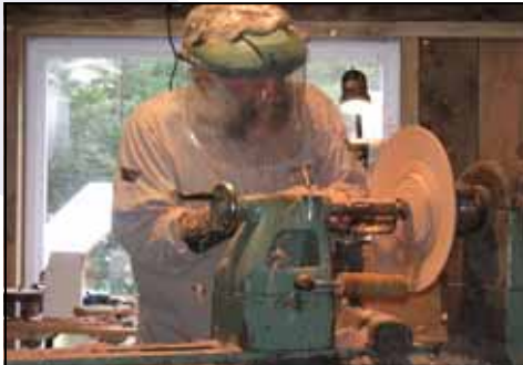
Taking down the rim to thickness. Get the rim thin before moving inwards to keep as much stiffness as possible under the gouge.
