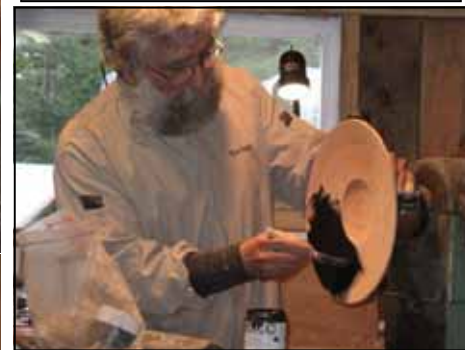
Applying black matt gesso as medium for carving design into rim. The bowl cavity will be finished after the "paint" dries for a crisp edge.
