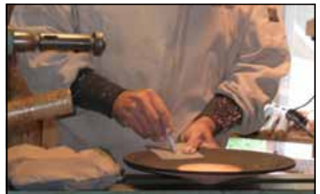
A very simple template is used to put a design on the surface. Al uses a watercolor pencil to put the design on the gesso. It is easier to erase its marks if you miss with the gouge.
