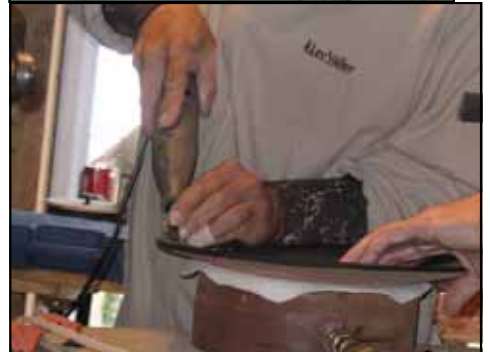
Using a vacuum chuck (and a helping hand) while carving the design.
