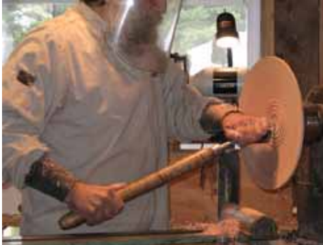
Applying black matt gesso as medium for carving design into rim. The bowl cavity will be finished after the "paint" dries for a crisp edge.
