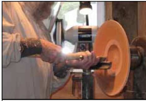
Forming the bowl cavity. Use calipers to keep from making the cavity walls too thin.
