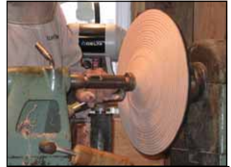
The bowl is reversed again using the tail stock and a padded jam chuck while the foot is being finished.
