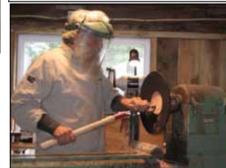
Final turning of the bowl cavity. A blunter bowl gouge is used to eliminate sanding the "painted" edge.
