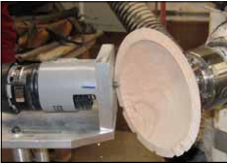
This is part of the setup Craig made to index a router used as a carving tool.
