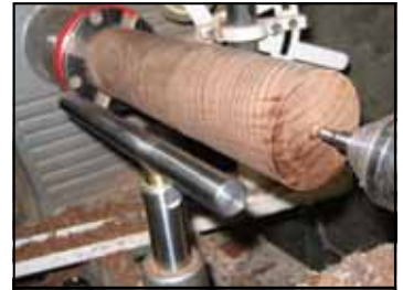
The straight, offset modular tool rest
