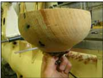
The iron forms a blue stain which streaks along the length of the wood fibers. Notice how these follow the same annual ring.
