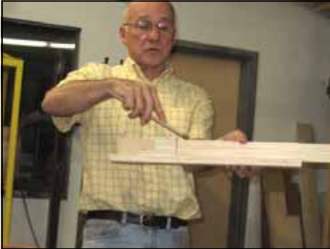
His 9 degree jig and hold down for the chop saw. He still has all 10 fingers.
