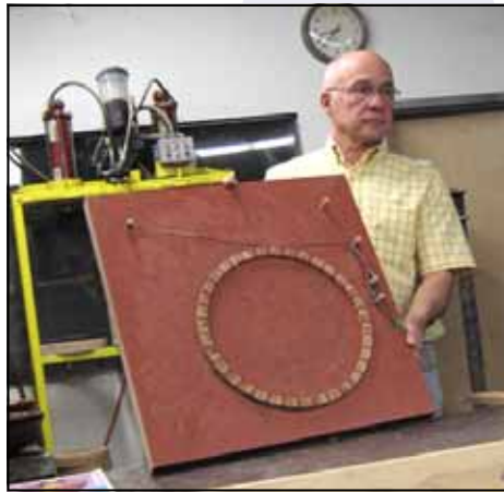
Here's a photo of Russ's flexible clamp for final ring assembly. A few wraps of string are wound around the piece and pulled to tighten.
