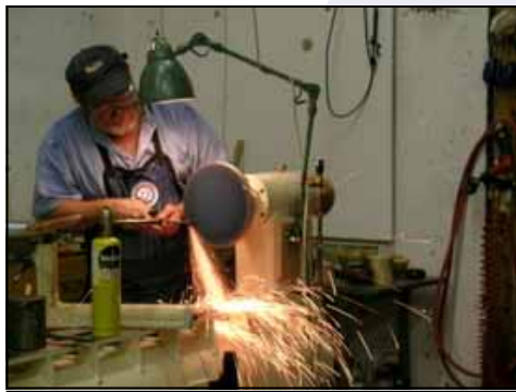
Alan grinding the initial shape into the hook tool blank on a homemade grinding disk - yet another application for the lathe.
