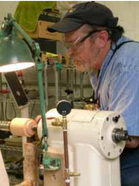
Alan makes a shoulder cut on a tenon for chucking the box blank
