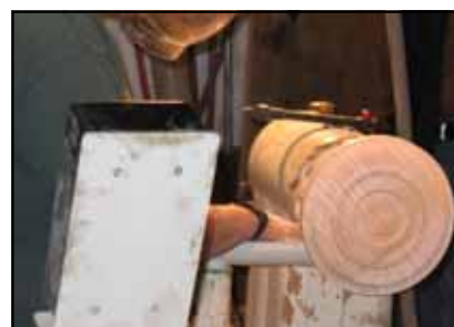
Working on the face side of the platter.
