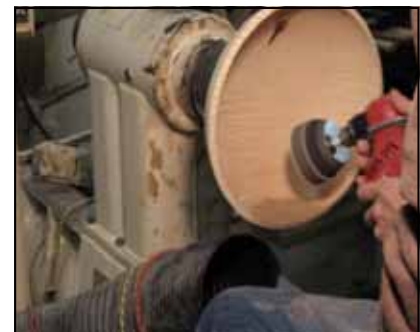
Sanding the inside, going from rim to center. Use the edge of the sandpaper which is moving in the direction of the grain.
