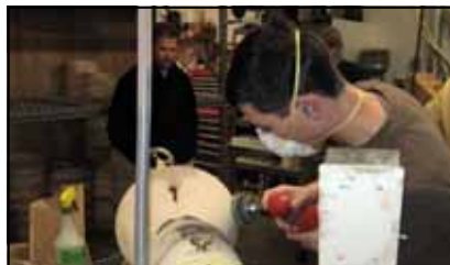
Sanding from bottom to edge sands with the grain on the outside of the bowl.
