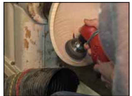
The bowl is rotated and a new quadrant is sanded from rim toward center.
