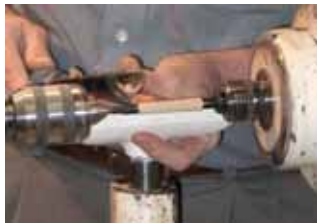
Dick's mandrel for this work is a center less, 2-piece, 1-blank mandrel.
