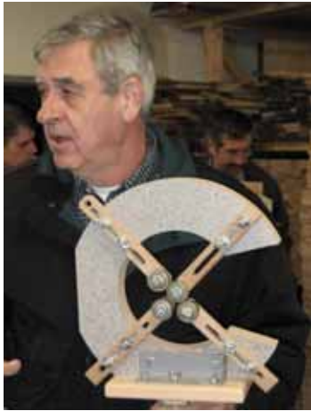
Herb Hurlbut- homemade steady rest,
