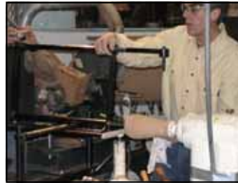
The Kelton hollowing rig with laser guide.
