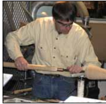
Deep hollowing with a very long handle for leverage.
