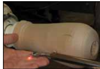
The laser is set to give a margin of about 1/4"
