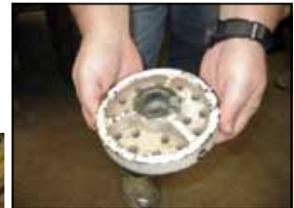
An unusual fault on a Oneway faceplate. The grub screw shattered the hub.
