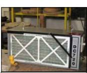
Hanging air filter—double furnace filters & quiet computer fans.
