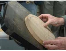
Cut on the outside of the line with the bandsaw. Make the cut coming in with the grainit will close up easier and less visibly. On the last line, on the extreme right in the drawing above, don't cut. It will be shaped on the lathe.
