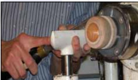
Shaping the exterior of the box.
