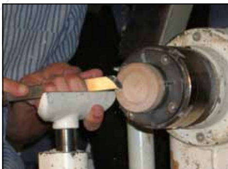
Rechuck and finish the bottom. Use a skew gouge for a fast, smooth finish.
