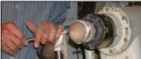
Jam the lid on using paper if lid is too loose. Finish forming the box with your favorite gouges, sanding, and final coats.
