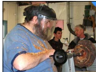
Coring a burl from the tailstock end. That's our Nova lathe.
