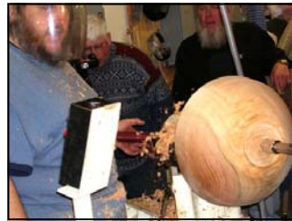
Coring out the outside bowl from the headstock side. He's using just one hand to guide the tool.
