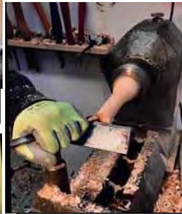
Remove tailstock and form a cup on the end.
