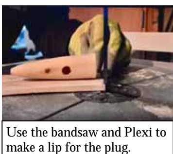
Use the bandsaw and Plexi to make a lip for the plug.
