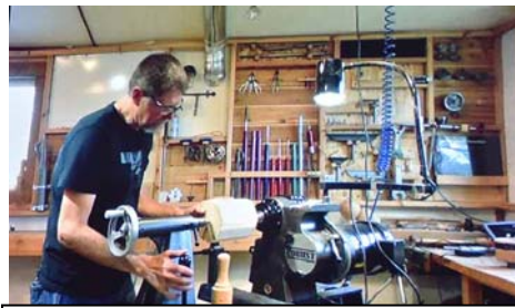
The block is mounted between centers.
