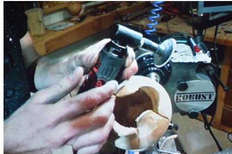
This is an air-powered 2" fine sander.
