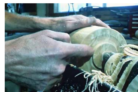
The tenon is sized for your chuck.
