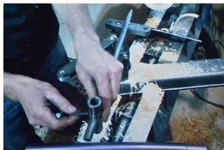
Trent is setting up his boring aid. It swivels and supports the bar, reducing fatigue.
