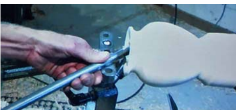
Using a curved tool to work close to the top of the cavity.
