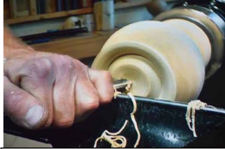
He starts center-boring the vase with a boring tool- borrowed from the gun making industry—photo on the right.
