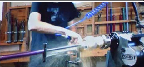
Trent uses compressed air to frequently clean out the cavity.
