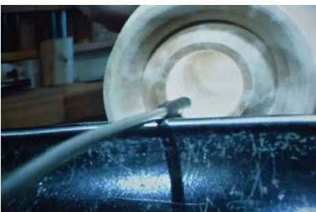
The cavity is enlarged and ready to have the walls thinned out. That's a fiber light looking into the cavity.
