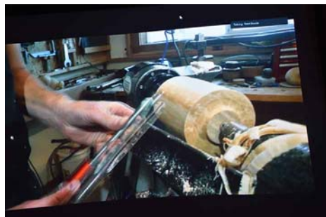
The cylinder is formed and a tenon is shaped on one end.
