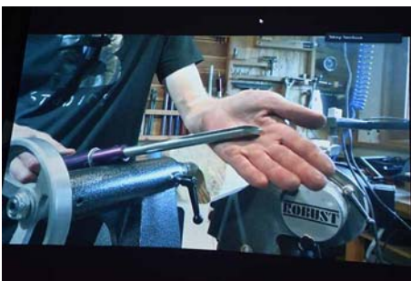
A normal gouge is used for the initial shaping of the cylinder.
