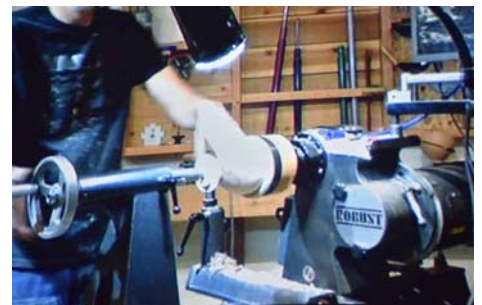
And Trent uses a vacuum chuck to hold the vessel while he turns the stem off the base and sands it smooth. He likes to sand a small flat spot on one side so it rest there and displays it as an artwork.
