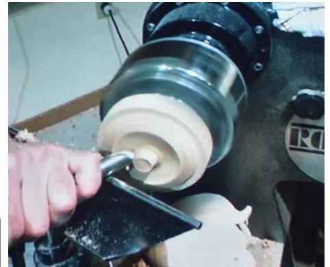
The plug is reversed into a jam chuck, thinned out as much as possible.
