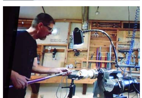
For this type of boring, use a long, heavy bar with a small, sharp tip. Do not try to take a fierce cut at the wood.
