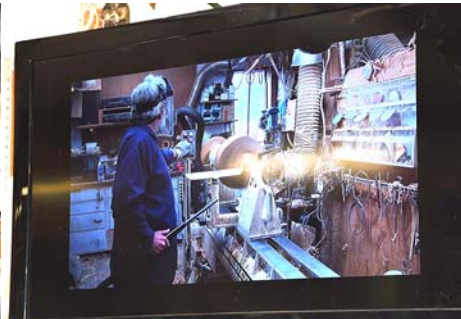
After rough cutting on a bandsaw, the blank is mounted on the lathe and the form of a bowl starts to emerge.
