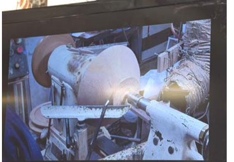
Another bowl is mounted using a vacuum chuck to finish the outside and base.
