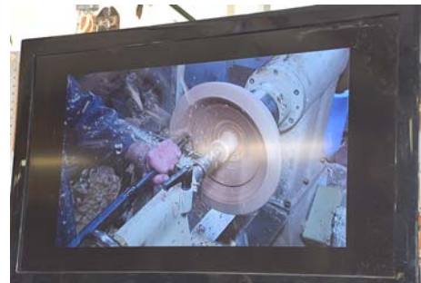
By using the tailstock, risk is reduced and big cuts on green wood reduce the lathe time.
