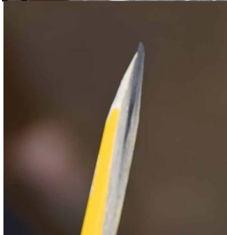
Janet flattens the lead on a #2 pencil so she can scribe a line accurately on a work piece.
