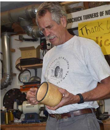
Harvie made several different vacuum chucks. This one has garage door skirting for a seal. It's wooden and needed several coats of varnish to reduce porosity.
