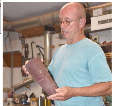
To form and sand the central hole he made this tapered sanding drum.
