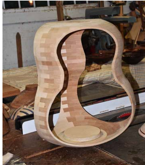
After constructing a circular body, he brought it to a sawmill to cut the guitar bodies out.
