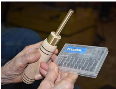
Dave also made a texturing tool using tiny bearings inside the brass tube.
