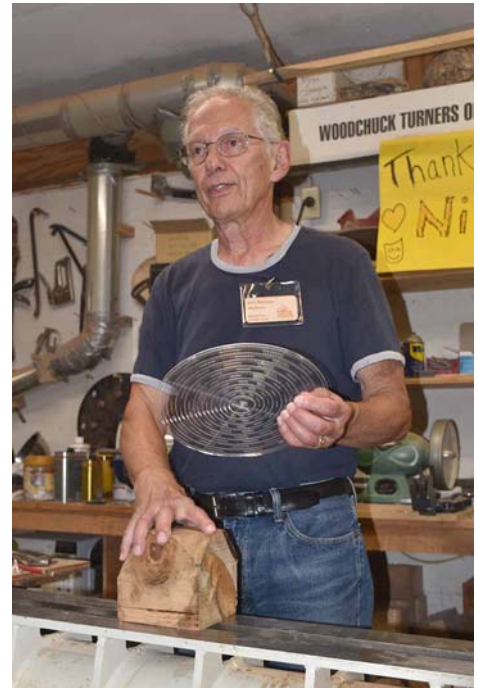
Barry uses a plexi circular guide to measure and mark the largest possible circle on a chunk of wood.
