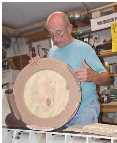
This is the fixture used to turn the bridges to the right radii to fit properly on the bodies.
