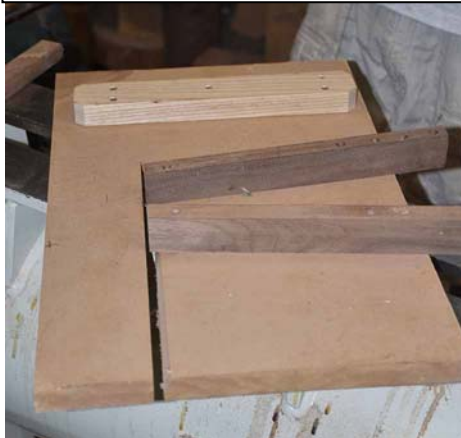
This is called a wedgie board. The two guides are symmetrical. To use it, put the cut piece against one guide, as shown in pic at far right, and cut. Roll it over, place against the other guide, cut again.
