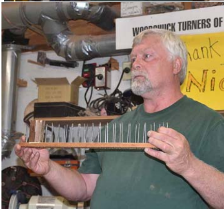
(Top) Brad reproduced a chart showing safe lathe speeds for various workpiece radii. (Bottom) He uses a board with large nails through it to group pen parts as he turns them.
