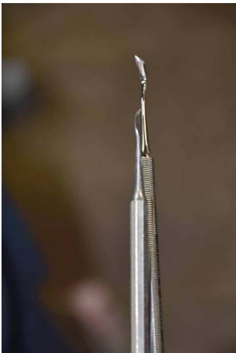
Dental tools can be sharpened and used many ways in woodturning. They make excellent scrapers and punches.
