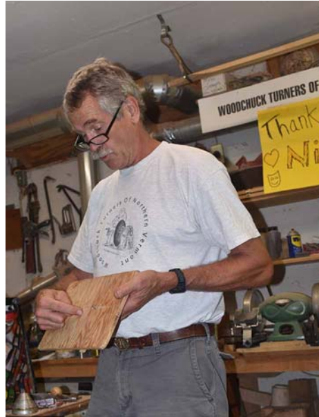
This board is used with a bandsaw to set the radius of a blank. Harvie holds a pin in one of several holes.
