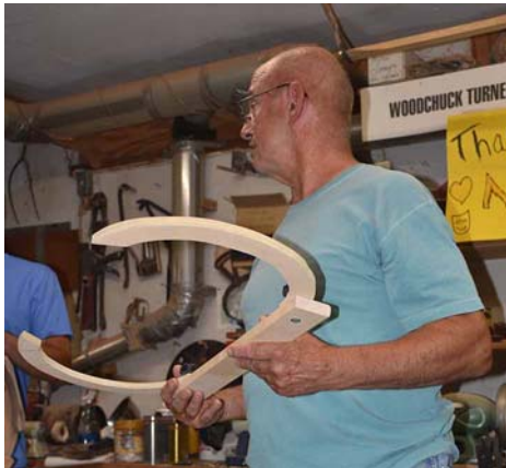
Here is the gauge he made to size the 3 sections of the guitar bodies.
