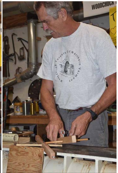
These devices are depth gauges for turning large bowls.
