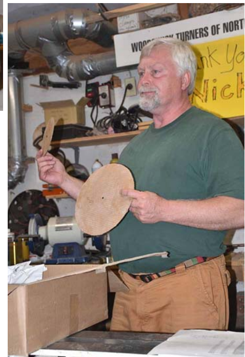
Cutting circles out of cardboard and labelling them as to size, lets Brad zing out round blanks on the bandsaw.
