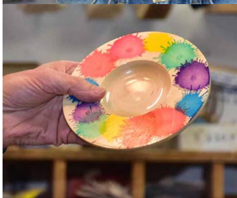
Dave has been experimenting with various types of decoration. Above, he's using multiple layers of spray paint, using dish-detergent as a "resist" between layers. Spray a base color and let it dry. Decorate that layer with painted-on soap. Spray another coat of color. Let it dry. Carefully wash the object down to remove the soap and the color remaining on the soaped part. The object on the lower left had dots of paint applied, and while still wet, blasted with air to leave splashes of color.
