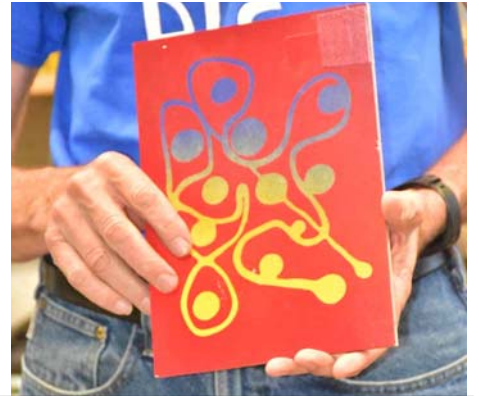
Dave has been experimenting with various types of decoration. Above, he's using multiple layers of spray paint, using dish-detergent as a "resist" between layers. Spray a base color and let it dry. Decorate that layer with painted-on soap. Spray another coat of color. Let it dry. Carefully wash the object down to remove the soap and the color remaining on the soaped part. The object on the lower left had dots of paint applied, and while still wet, blasted with air to leave splashes of color.
