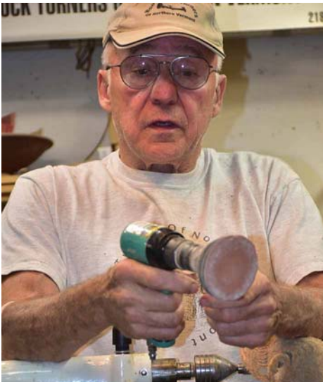
For finish sanding, Russ will use a very fast air-powered sander.
