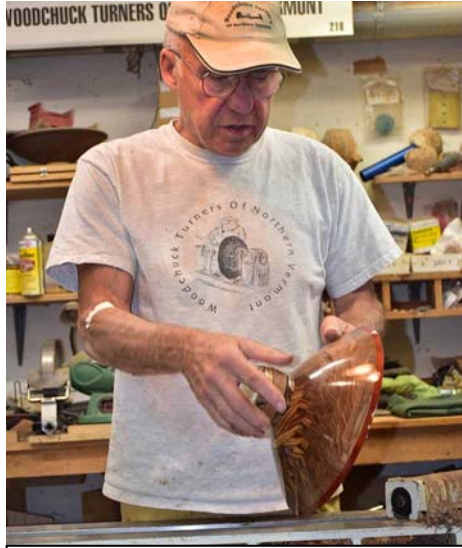
When Russ wants a gloss finish, he may seal the surface with a spray of shellac, then apply wipe-on poly.
