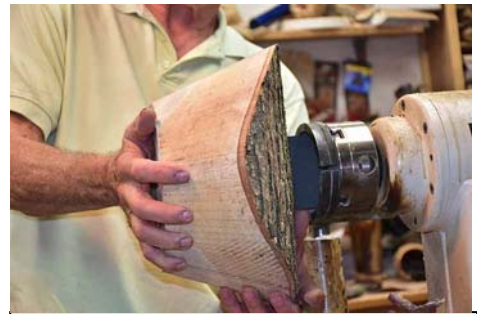
This is a big driver for roughing out large bowls. It is clamped in position in the jaws of a 4-jaw chuck. Bring the tailstock up and adjust position to center and balance the back of the stock.
