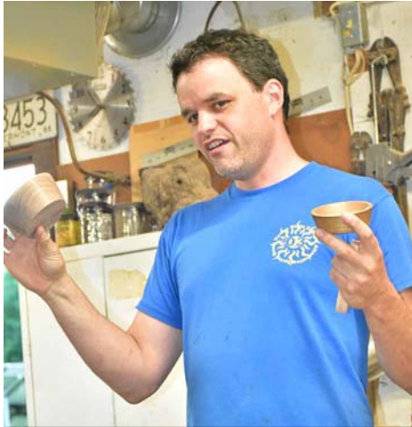
Nick tackles some multi-piece jobs. Here are 2 “saucers” which will be attached to the bases of wine decanters by Simon Pierce Glass. Nick developed jigs and fixtures to allow him to repeat each task and end up with near identical results each time.
