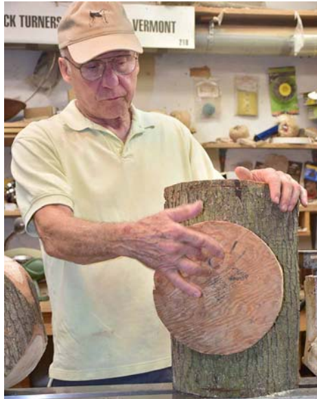
Making templates of various sizes allows you to get the largest blank out of a log. Nail the template to the round side and bandsaw around it.
