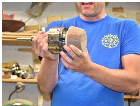
This jig is attached to the live center and holds the wood—after a preliminary cutting of a vacancy—to register the piece into a vacuum chuck.
