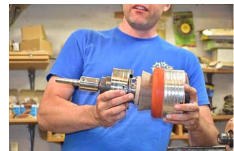
By registering the piece in the vacuum chuck and removing the jig, Nick can finish turning the interior and get a good, concentric rim and depth.
