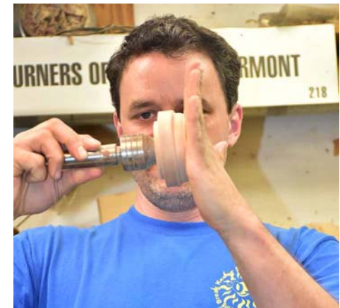
This jig allows Nick to set the depth of the cut.
