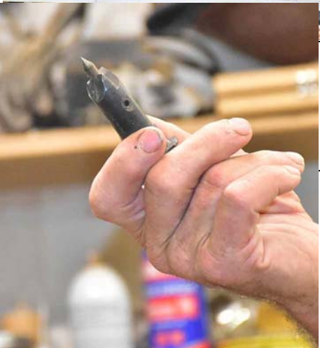
These are 2 other mounting options. For security, drill a same-size hole into good solid wood especially through bark. These mounting methods pretty much preclude shifting the back end of the stock for better centering.
