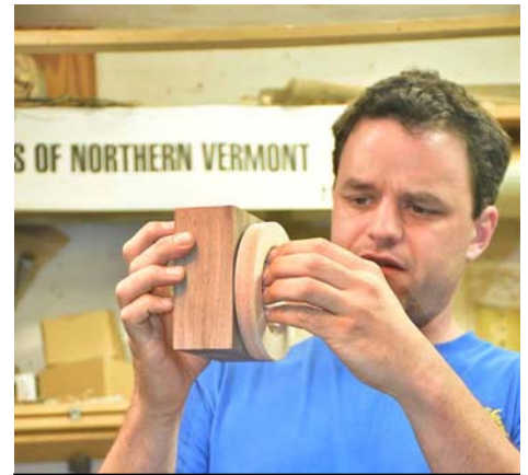
The first fixture mounts in a chuck and sets the large diameter of the saucer.
