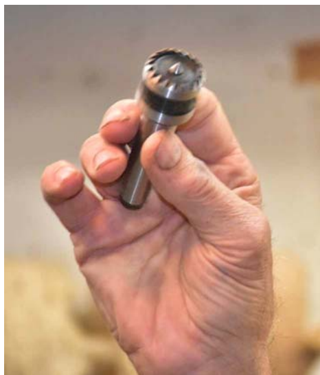
These are 2 other mounting options. For security, drill a same-size hole into good solid wood especially through bark. These mounting methods pretty much preclude shifting the back end of the stock for better centering.
