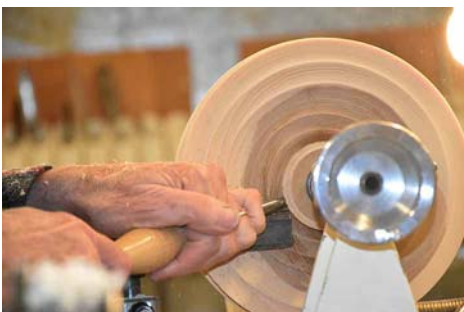
Thinning down the round to start forming the intermediate branches.
