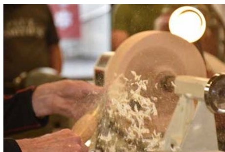
Working the outer edge to form the lowest branches & the “trunk” of the tree.
