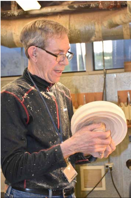
Reversing the workpiece to do the reverse side.
