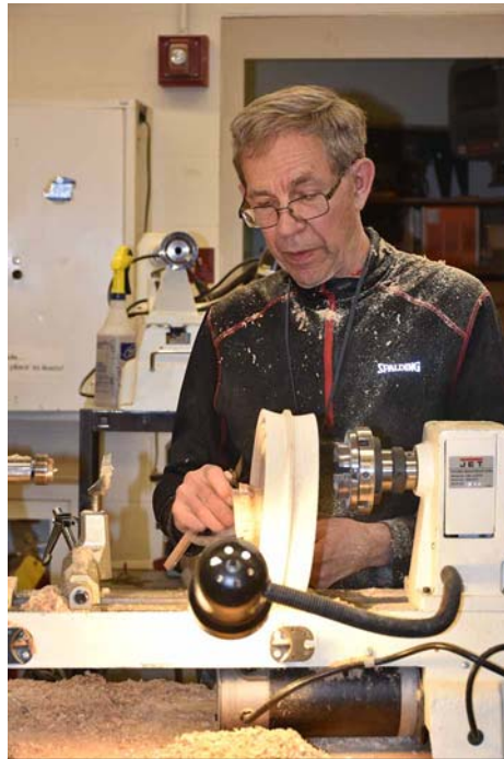
Attaching the tenon to the chuck.
