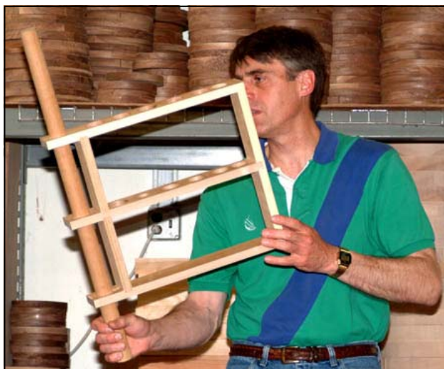
Craig shows a shop-made tool holder for his lathe.
