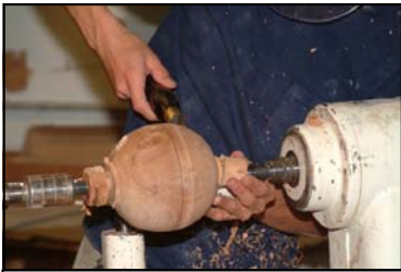
Parting off the tenons
