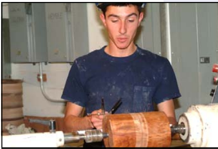
Proportioning the workpiece
