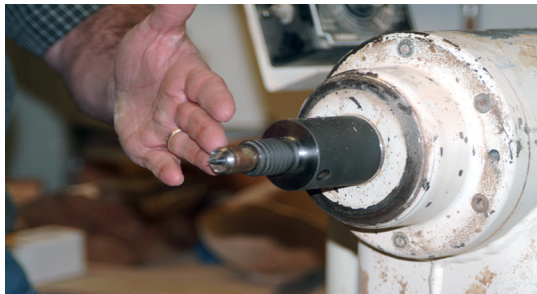
Using a dead center as a live, spurless center for safety
