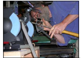
Setting up with the Wolverine jig; spindle gouge
