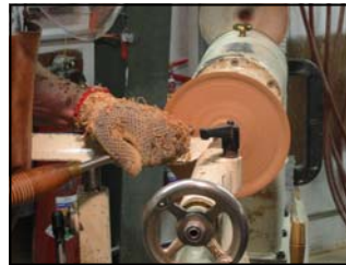
Deepening the cavity with bowl gouge
