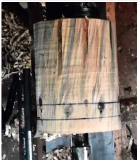
This line shows where to cut to take advantage of the whole branches.
