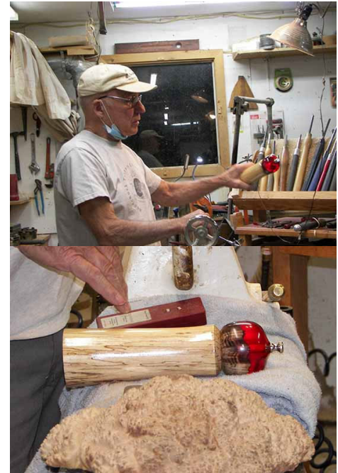
Russ has experimented with using clear epoxy as a turned element. Here, the knob on his pepper mill is a section of burl encased in epoxy to show the texture.
