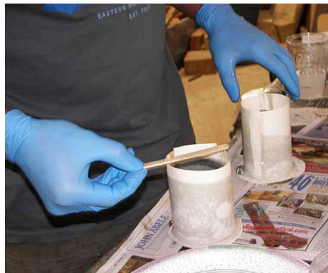
Andy adds a 2nd layer to an object. The form is heavy paper and will be turned off.
