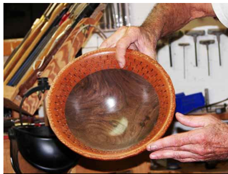
A variation of segmented turning: A solid walnut bowl gets a pierced-segmented rim.
