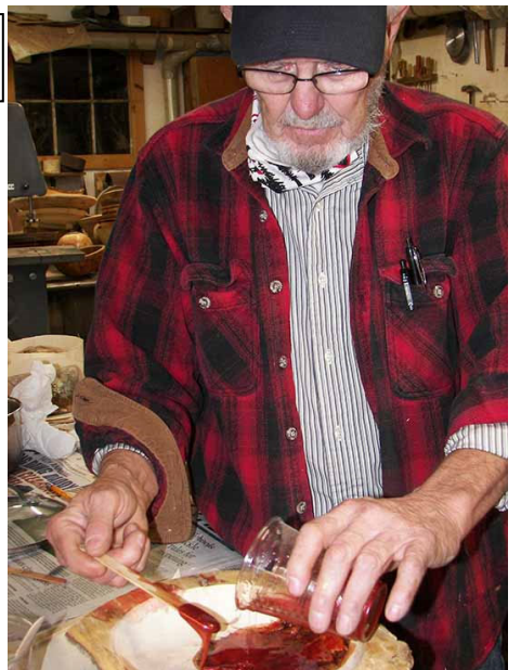
Brad adds some more and spreads it around. The epoxy will seep into all the crevices.
