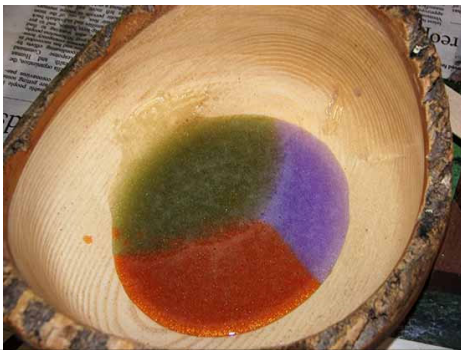
After the epoxy sets, Karen will have 3 distinct colors filling the bottom of this natural-edge bowl.
