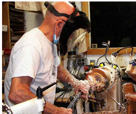
Brad dumps any excess epoxy into a container and when it's full, he might turn it down to see what he can get from it. Here, Russ goes to work on one of the dump-clusters.
