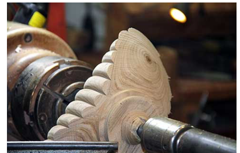
Make a tenon to fit your scroll chuck on the base.
