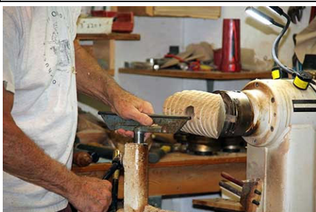
Re-mount the workpiece and start to hollow the top.
