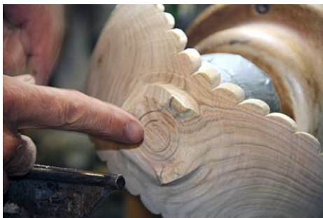
Before final finishing, this is what the footed bottom looks like.
