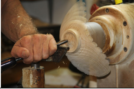
The bowl is reversed onto a vacuum chuck and the base hollowed out.
