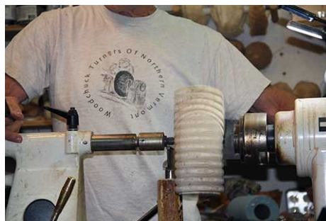
The cylinder is re mounted between centers to start forming the back of the oval.
