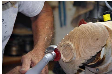
Russ marks out 3 equally spaced feet on the base and cuts away the waste with a small grinding tool.
