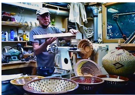
This board has a strip of sandpaper on it. It's used to flatten each ring before gluing the next one on.
