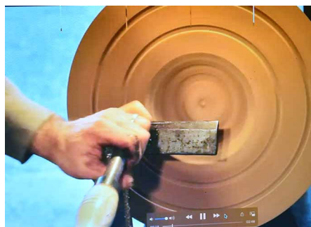
Coring. First, define the cuts- 3 or more total bowls.
