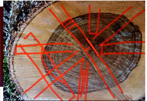
Diagramming quarter-sawn vs. rift-sawn. Mike uses quarter-sawn oak for platters.
