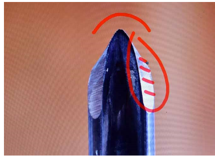
This is an ideal grind for a bowl gouge. Even angles.
