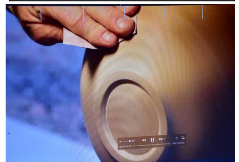
The bowl has been reverse mounted on the vacuum chuck and the bottom shaped. Final fine sanding.
