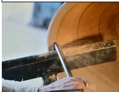
Thinning out the inside of the bowl, using a shear scraping cut.
