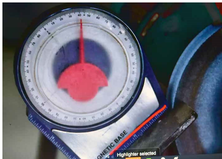
Mike sets the flat tool rest for about 42 degrees.
