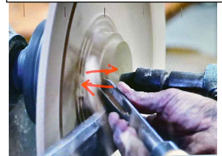
Reducing the front tenon. The tail-stock stays for safety to the last.
