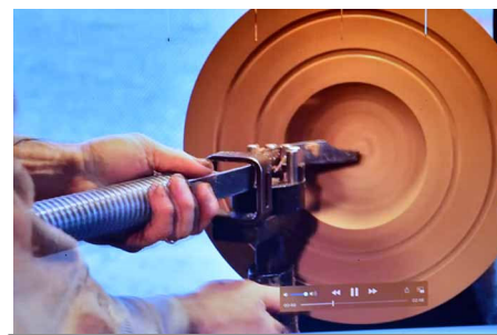
Set up the McNaughton rest so the tool will swing to near the center.
