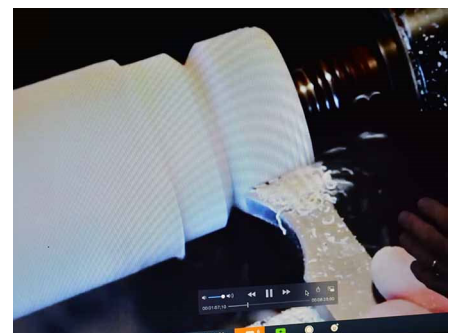
And threading the male end. Note the undercut.
