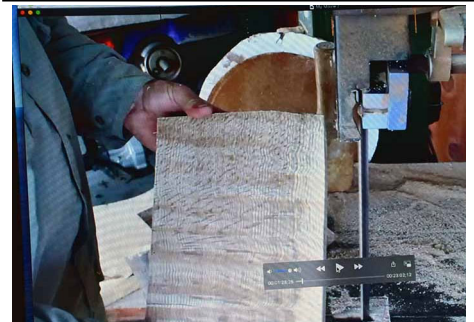
Carving out a quarter-sawn slab on the bandsaw
