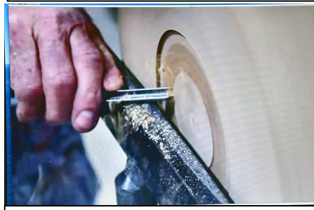
Hollowing a recess for the chuck.
