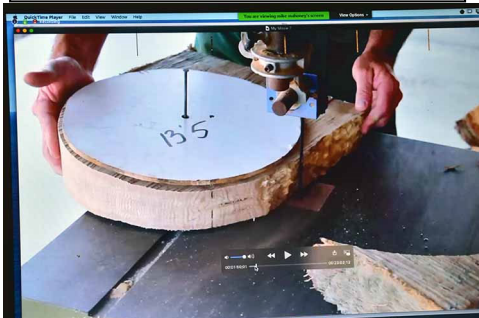
Using a template and the bandsaw to create rounds from a slab.
