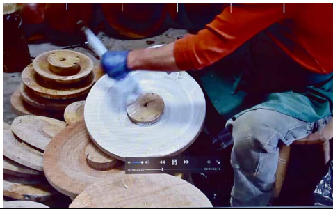
Coating the rough platter with "Elmer's Glue" to dry slowly.
