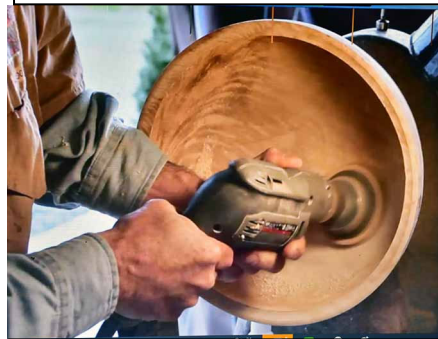
Power sanding the interior.
