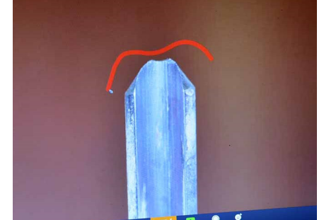
Very poor grind. Can't control the cut.
