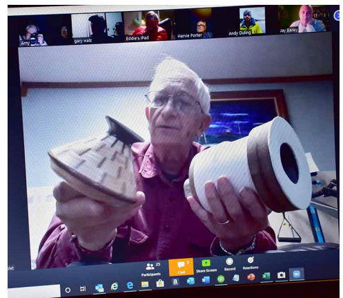
Mickey Palmer uses PVC pipe and dense foam, among other items, to make custom vacuum chucks. His design uses a single base and several top fittings.
