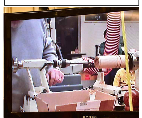
Next, using a 1-1/16" bit, drill about half-way through the blank.
