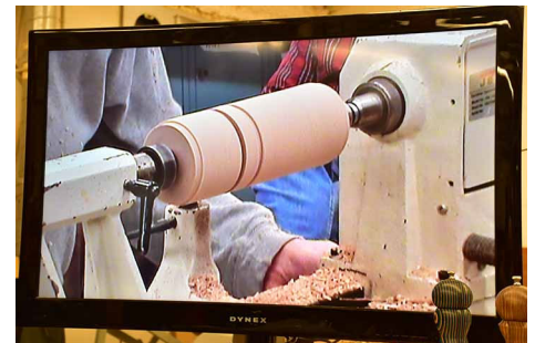
The blank is divided into the top, the top of the bottom, and the bottom length. A tenon is turned on each end to fit a 4-jawed chuck.
