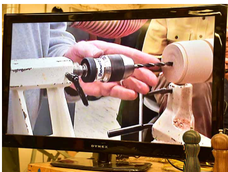
A (roughly) 1/4" hole is drilled through the top and into the bottom part.
