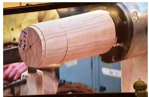
The top is friction-fit to the bottom so the finish shape is flowing between the 2 pieces.
