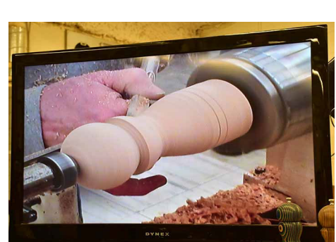
Sanding the final shape. Finish will be applied and then the mechanism screwed into the body.
