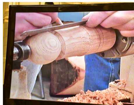
Measuring the placement of the character lines.
