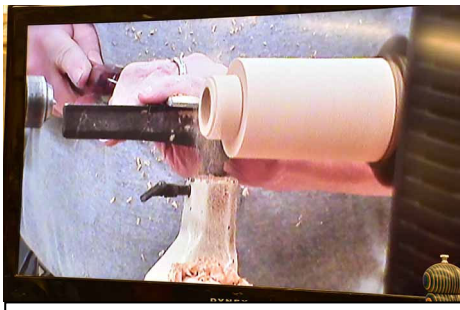
Turning the top of the bottom to fit into the recess in the top. Go slow and try many times. You want a frictionless tight fit when done.
