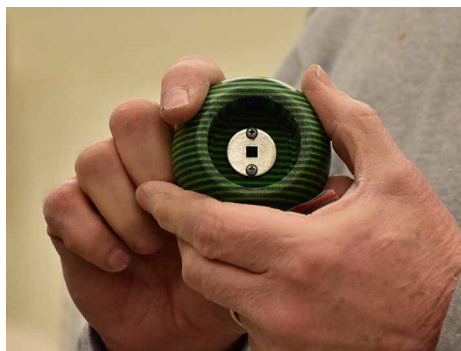
The Chef Specialties unit puts the nut which turns the shaft up into a recess in the top.
