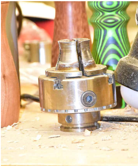
This is the chuck Brad uses to allow for tool work the full length of the peppermill.
