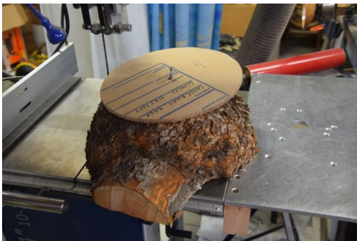
Preparing to bandsaw one chunk into a circular blank.
