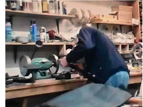
Here, Dave demonstrates sharpening the gouge using the Ellsworth jig and the Oneway Wolverine fixture.
