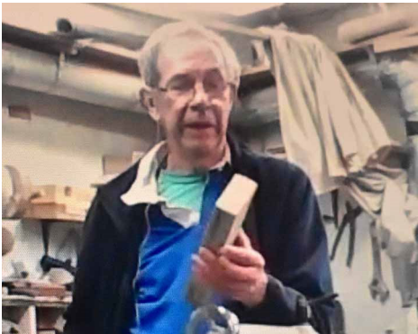
Dave uses a simple, portable gauge to set the length of his Ellsworth bowl gouge. It has holes drilled to 1-5/8" and 2" with a penny glued at the bottom.
