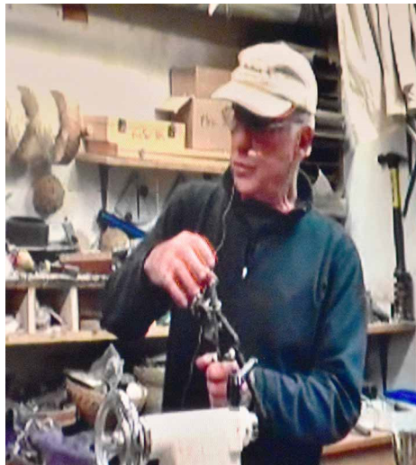
Russ talks about setting up a gouge for sharpening with the Oneway jig system. Use a depth block to set the jig onto the gouge. The setting block should be 1-5/8" to 2" deep. The angle of the jig's leg will vary the amount of sweep on the cutting edge.
