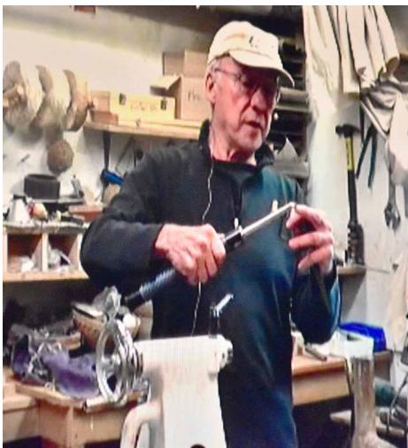
Russ talks about setting up a gouge for sharpening with the Oneway jig system. Use a depth block to set the jig onto the gouge. The setting block should be 1-5/8" to 2" deep. The angle of the jig's leg will vary the amount of sweep on the cutting edge.
