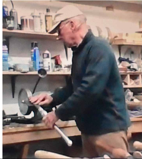
Russ explains the spindle roughing gouge. The blade should be straight across. It can be sharpened using the Oneway jig and rotating it evenly, spinning it using the heel as the focal point or use the flat rest set at the proper angle. Either way, grind a smooth bevel from ear to ear of the tool.
