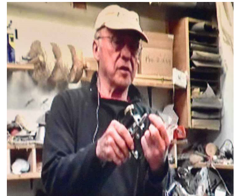
Russ talks about setting up a gouge for sharpening with the Oneway jig system. Use a depth block to set the jig onto the gouge. The setting block should be 1-5/8" to 2" deep. The angle of the jig's leg will vary the amount of sweep on the cutting edge.
