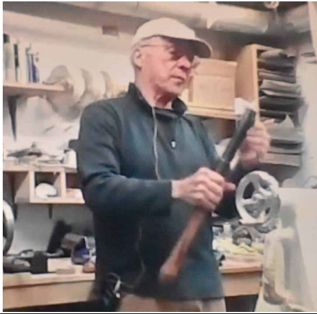
Russ explains the spindle roughing gouge. The blade should be straight across. It can be sharpened using the Oneway jig and rotating it evenly, spinning it using the heel as the focal point or use the flat rest set at the proper angle. Either way, grind a smooth bevel from ear to ear of the tool.
