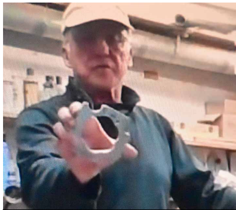
This is a gauge with many of the angles needed to set the geometry of the tool rest on the grinder and other needed angles.
