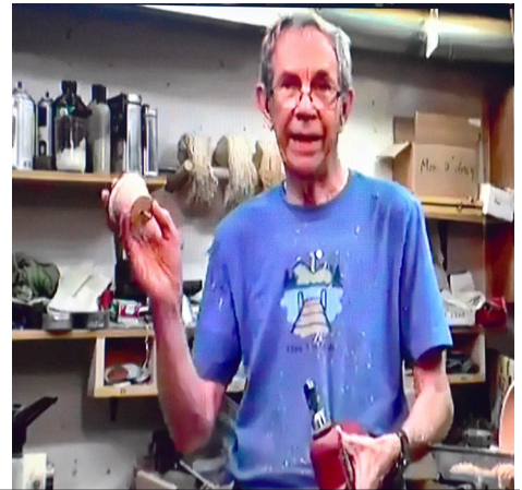
Dave uses a drill gun and specially made sandpaper holders. Rather than strip the sandpaper off the backer each time, he has the several grades mounted on separate holders. This extends the life of the sandpaper.
