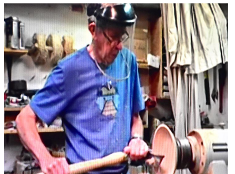
First, a bottom is formed on the outside complete with a tenon to fit the drive chuck.
