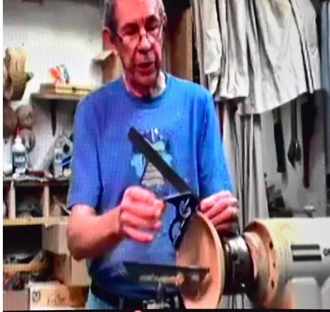
The bowl is hollowed. The rim is measured to be flat. The bowl is then brought to the desired thickness with the rim having enough width to take 1/4" reeds.
