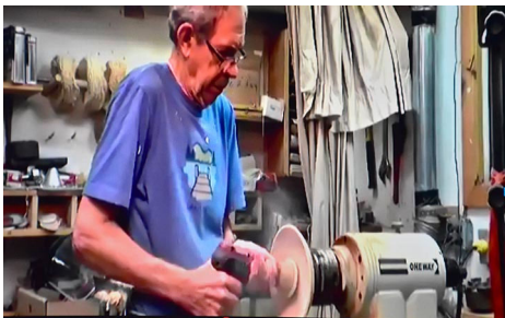
The bowl bottom is thoroughly sanded before drilling holes evenly spaced around the rim. It appears that there may be 15 holes in this example.
