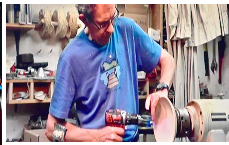
The bowl bottom is thoroughly sanded before drilling holes evenly spaced around the rim. It appears that there may be 15 holes in this example.
