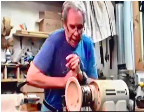
First, a bottom is formed on the outside complete with a tenon to fit the drive chuck.
