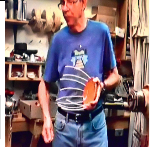
Dave uses a drill gun and specially made sandpaper holders. Rather than strip the sandpaper off the backer each time, he has the several grades mounted on separate holders. This extends the life of the sandpaper.
